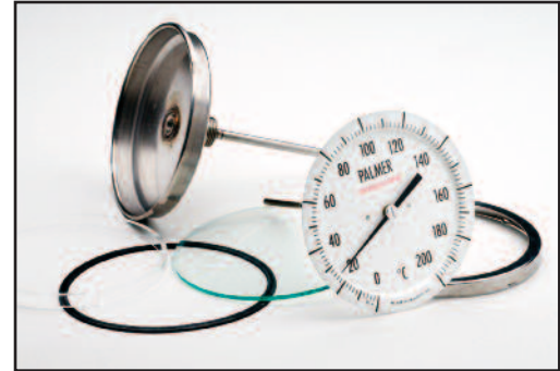
Disassembled replaceable element bimetal thermometer.
